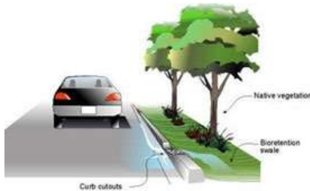
Figure 3- Stormwater runoff from surrounding area draining into bioswale. Adapted from Guillette (2010).
