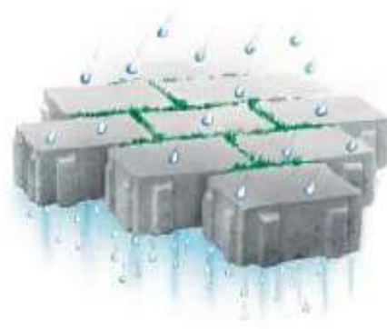
Figure 4-Water infiltrating through permeable pavements into the soil below. Adapted from Dierkes et al. (2002).
