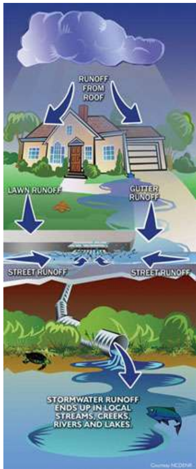
Figure 1- The basic flow of runoff after a rainfall. Adapted from City of Wilmington (2009).
