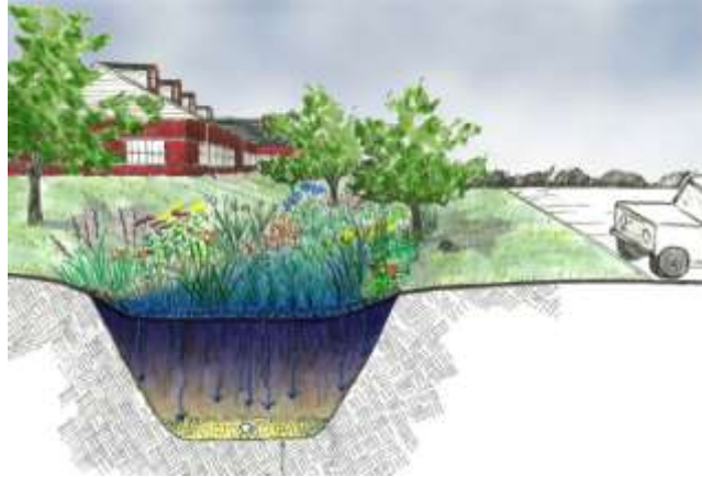
Figure 5-Typical bioretention garden in which runoff infiltrates into the soil. Adapted from Griffin (2008).
