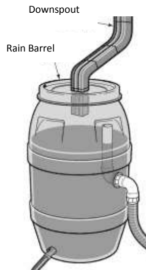
Figure 7- Stormwater flows from roofs of adjacent building and then retained in the rain barrel. Adapted from WATER (2011).
