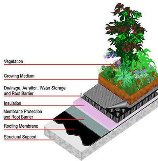
Figure 6- Layers found in a green roof system, which allows for precipitation to infiltrate. Adapted from Roof Helper (2011).
